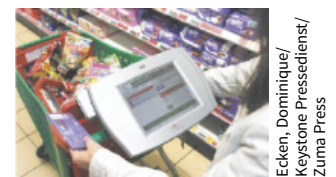
FIGURE 8.7 Small RFID reader and RFID tag.
