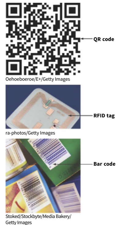
FIGURE 8.6 Bar codes, RFID tags, and QR codes.
